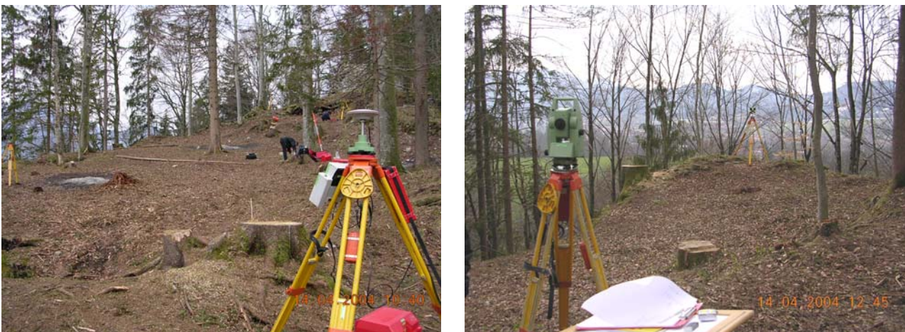
Fig. 5: Impressions from the geodetic measuring campaigns at the plateau area of the Hohenburg; left: GPS receiver Leica System 500, right: tachometer Leica TCR System 700
