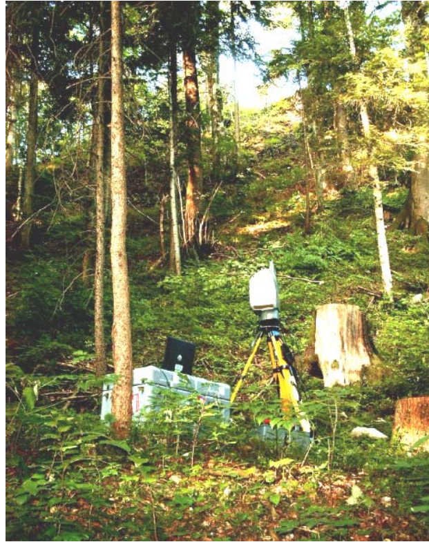
Fig. 6: Laser scanner Leica HDS 3000 at the western flank of the castle bedrock
